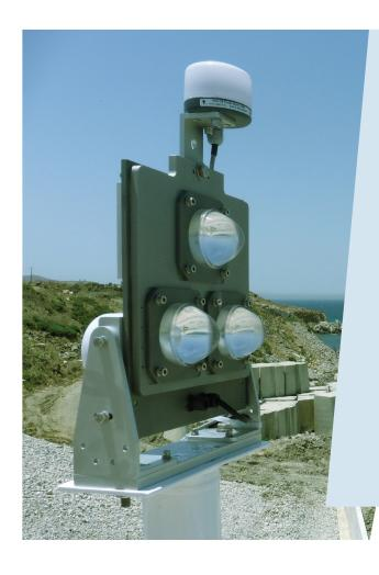
The VRL-74 operates at high intensity, making it suitable for use as a lead or range light. With low power consumption and LEDs that require no maintenance, it is an ideal choice for sites that are remote and solar powered. It can achieve a night range up to 22NM @ 0.74T.
